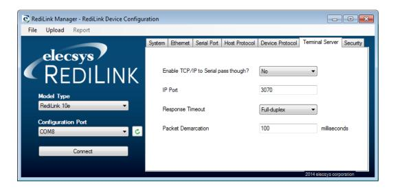
The Terminal Server may be used, for instance, when a remote host needs to connect its configuration utility directly to a PLC, bypassing the Host and Device protocol polling options of the RediLink. The Terminal Server serial port can be used simultaneously with the serial Device Protocol polling, as long as the connected device is able to accept both polled and pass-through messages interchangeably.
