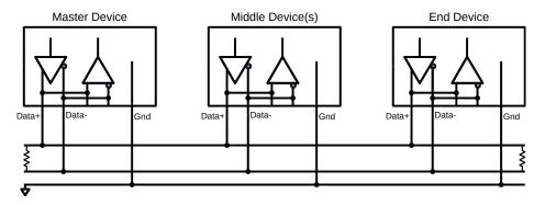
4-wire to 2-wire RS-485 Device Connections
