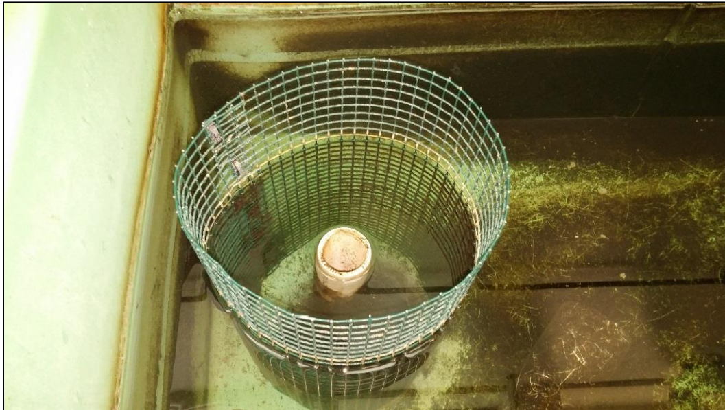
Figure 4. Overflow pipe and hardware cloth cylinder. The overflow pipe limits water depth to a maximum of 13 inches. During water exchanges, the pipe is removed manually from the drain opening to allow approximately 3 to 4 inches of water to drain from the tub. The hardware cloth cylinder allows particulate debris and animal wastes to accumulate at the base of the overflow pipe for subsequent flushing from the tank during water exchanges. In Figure 3 above, note the presence of weights positioned atop the cylinder. The pressure applied to the cylinder by these weights prevents frogs from passing under the cylinder and near the overflow pipe.
