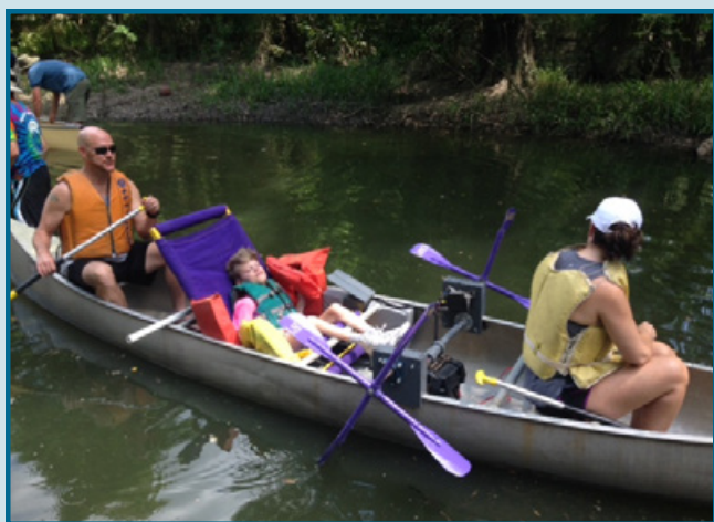
Canoeers put the new adaptive paddling device to the test on its maiden voyage. The battery-operated unit operates by pushing a button that spins dual 4-paddle wheels in a forward motion, helping to propel the canoe.
