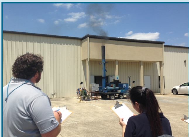
During the smoke test, LDEQ environmental scientists mark an opacity reading as black smoke emanates from the smoke generator at the LDEQ warehouse in Port Allen.
