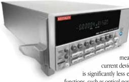
With eight current measurement ranges and high speed autoranging, the Model 6487 Picoammeter/ Voltage Source instrument can measure currents from 20fA to 20mA, take measurements at speeds up to 1000 readings per second, and source voltage from  $200\mu$ V to 505V. Its 10fA resolution, superior sensitivity, voltage sweeping, and Alternating Voltage resistance measurements make it well suited for characterizing low current devices. Using the latest current measurement technology, it
