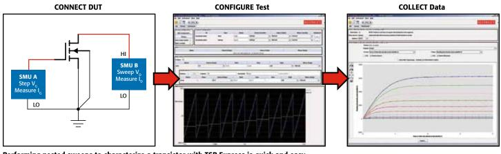
Performing nested sweeps to characterize a transistor with TSP Express is quick and easy. Data can be exported to a .csv file for use with spreadsheet applications such as Excel.
