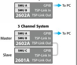
TSP-Link, a high speed system expansion interface, makes it easy to scale the system's channel count to match the application.
