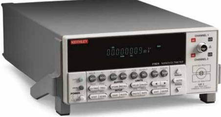
The two-channel Model 2182A Nanovoltmeter is optimized for making stable, low noise voltage measurements and for characterizing low resistance materials and devices reliably and repeatably. It provides higher measurement speed and significantly better noise performance than alternative low voltage measurement solutions.
