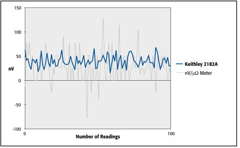
Compare the Model 2182A's DC noise performance with a nanovolt/micro-ohmmeter's. All the data shown was taken at 10 readings per second with a low thermal short applied to the input.
