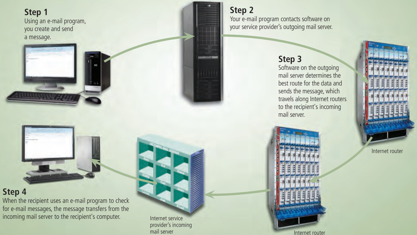
Figure 2-27 This figure shows how an e-mail message may travel from a sender to a receiver.
