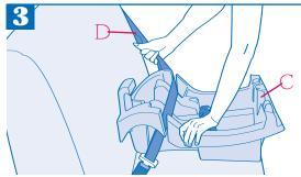
Push down on the base C while pulling the shoulder belt D tightly to remove all slack from the lap portion of the belt.
