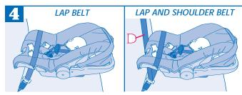
**NOTE:** In vehicles with a lap and shoulder belt D and a free sliding buckle tongue, and emergency locking retractors (ELR) you must install with the locking clip. Unless your vehicle owner's manual provides otherwise. See "Using the Locking Clip" on page 23.
