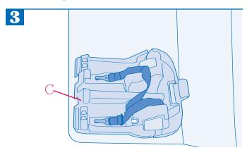
When the LATCH system is not in use, you **MUST** securely store it in the area provided in the base  $\mathbb{C}$ . Fold the harness strap, place it in the middle, and put the hooks in the slots located on each side of the storage area. A loose LATCH harness and hook may injure your child.
