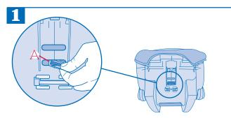
To reposition the crotch strap, turn the harness anchor A on the end of the crotch strap sideways and push it through the slot in the restraint seat.
