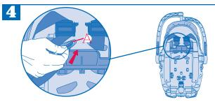
Choose the appropriate slots for the new harness position. Push the harness anchor A, buckle tongue, and harness strap and chest clip through to the front of the child restraint. Repeat for the other harness strap. **NOTE:** Harness strap should start at or below the child's shoulders.
