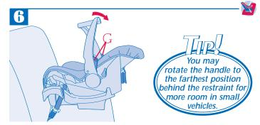
Rotate the handle to the down position by pressing on the red handle triggers G located on each side of the child restraint. Move the handle back until it locks into place behind the child restraint. Place the child in the restraint and secure.
