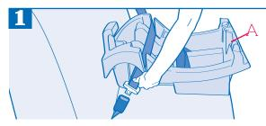
Secure the base A to your vehicle seat by routing the vehicle seat belt through the openings on the sides of the base. You may also let the vehicle shoulder belt fall against the vehicle seat back. Be sure that the vehicle shoulder belt does not lie inside any portion of the convenience base.
