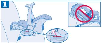
After securing the infant, place the restraint into your vehicle. Adjust the restraint so that the level line  ${\boldsymbol A}$  is parallel with the vehicle floor.
