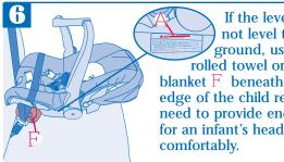
If the level line A is not level to the ground, use a tightly rolled towel or small blanket F beneath the front edge of the child restraint. You need to provide enough recline for an infant's head to lie back
