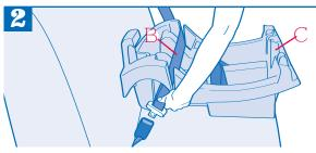
Thread the seat belt B through the base C (or child restraint) and buckle the seat belt.
