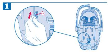
Push the harness anchor A located on the back of the child restraint through the slot to the front of the seat shell. Repeat this procedure on both sides.
