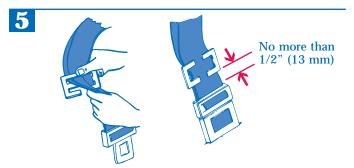
Thread both straps of the seat belt onto the locking clip, and slide into place.
