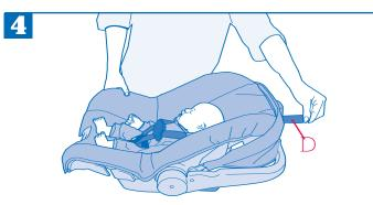
Tighten the harnesses by pulling on the harness straps D from the back of the harness adjusters.
