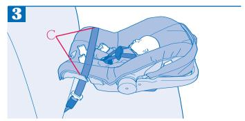
Secure the restraint to your vehicle by routing the vehicle seat belt through the belt slots  $\boldsymbol{C}$  on the sides of the restraint.
