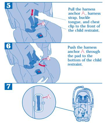
Pull the harness anchor  $\boldsymbol{A}$  through the bottom of the child restraint, and clip into place. Repeat on the opposite side.
