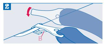
Press the tab  $B\,$  on the hook. Press hook in and twist to release. Repeat on other side.
