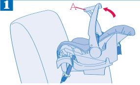
Move the handle A to the up position by pressing the handle triggers and rotating the handle until it locks into place above the child restraint.
