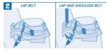
**NOTE:** In vehicles with a lap and shoulder belt **and** a **free-sliding buckle tongue**, you **MUST** install with the locking clip. See "Using the Locking Clip" on page 23.
