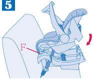
Secure the infant restraint to the base by placing the front of the seat under the hook F and snapping into place.
