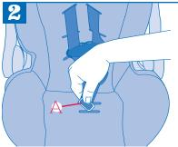
Insert the crotch strap anchor A into the slot that is the closest to the child **AND** the most comfortable for the child.
