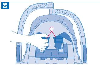
To loosen the harness straps, squeeze the harness adjusters  $\boldsymbol{C}$  while pulling on the straps from the front of the seat.
