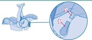
Guide each end of the canopy strip A into the canopy holders B located on each side of the child restraint.
