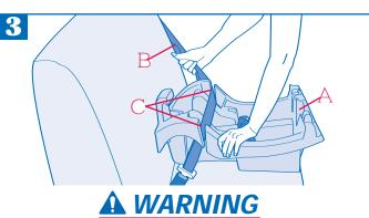
**DO NOT** use this child restraint if it moves more than 1 in. (25 mm) forward or side-to-side at the seat belt path. Serious injury or death may occur. Move the child restraint to another seating location, or try to tighten the seat belt again.
