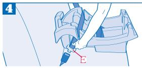
Hold the lap and shoulder belts together just behind the free sliding buckle tongue E and unbuckle the seat belt.
