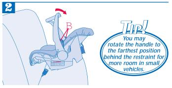
Rotate the handle to the down position by squeezing both handle triggers  $\ensuremath{B}$  .
