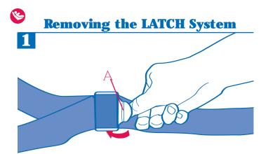
Tilt and slide the adjuster A to loosen.
