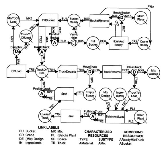
Figure 3 Process model for concrete placement.
