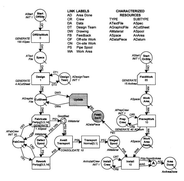
Figure 1 Pipe-spool process model.
