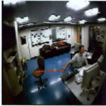
Figure 2: The last frame of a 30 frame sequence with five trajectories identified. Four nearly stationary trajectories were found (one on the person's head, one on the person's hand, one on the couch in the background, and one on the door in the background). The final trajectory resulted from the chair being pushed across the floor.
