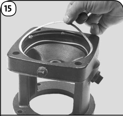
Clean the recessed areas in the motor stool that will hold the seal ring and outer sleeve gasket. Lubricate them with an FDA-approved lubricant. With the ends pointing down, fit the corrugated spring (60) into its recessed area. Spring must be positioned as shown—tips pointing downward and toward 1/4" plug.
