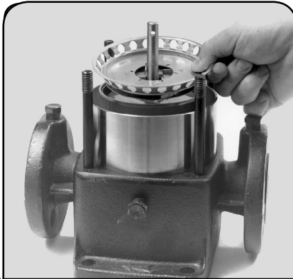
Fit the outer sleeve (55) over the impeller stack and press the top guide vane (50a) or top plate (50b for CR4 only) into place on the top chamber.
