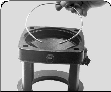
Clean the recessed areas in the motor stool that will hold the seal ring and outer sleeve gasket. Lubricate them with an FDA-approved lubricant. With the ends pointing down, fit the corrugated spring (60) into its recessed area. Spring must be positioned as shown—tips pointing downward and toward 1/4" plug.
