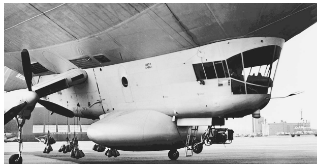
FIGURE 2. Navy blimp installation of the AN/APS-70 radar. The radome appears at the bottom of the blimp.
