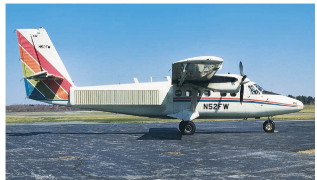
FIGURE 7. MASR antenna mounted on the side of a DeHavilland Twin Otter aircraft. The antenna measures 15 ft \times 2.5 ft \times 5 in and weighs 370 lb.
