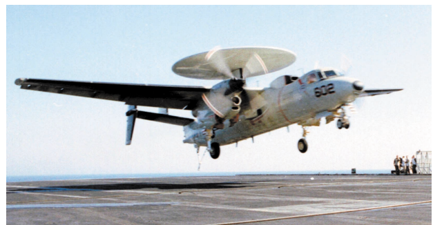
FIGURE 5. The E-2C Hawkeye aircraft shown returning to its carrier from a mission. With its displaced-phase-center antenna (DPCA) overland radar, the aircraft can track more than 2000 targets at once and monitor three million cubic miles of airspace.
