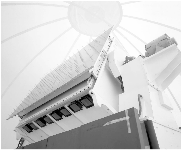
FIGURE 13. Photograph of hexagonal-spaced 96-element test array inside the radome of the far-field antenna measurement range. The array has a total of 192 elements, but the outer two rows around its circumference are terminated with matched loads to reduce boundary effects on the antenna patterns.
