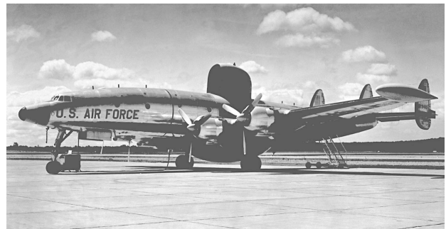
FIGURE 4. AN/APS-95 radar installed in a modified Lockheed Super Constellation aircraft.
