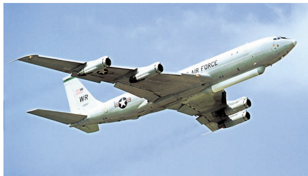
FIGURE 10. Air Force Joint Surveillance and Target Attack Radar System (Joint STARS) aircraft. Note the DPCA antenna mounted forward under the fuselage. Image courtesy of Northrop Grumman Corporation.
