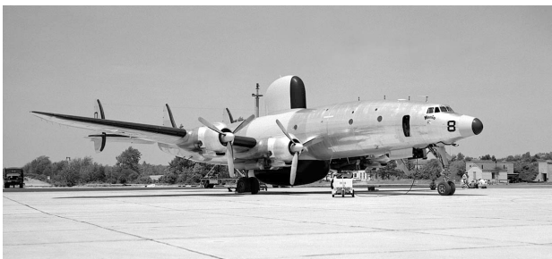
FIGURE 1. The WV-2 aircraft, an original carrier of the UHF AN/APS-70. A 17 \times 4 -ft antenna is mounted below the aircraft inside the black radome.
