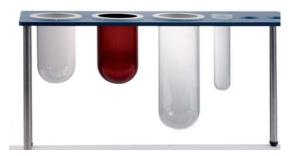
(Left to right) 1L TruAlign vessel, 1L low actinic - red TruAlign vessel, 2L TruAlign vessel and 200 mL TruAlign vessel
