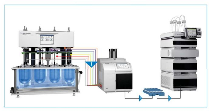
Samples collected by the 850-DS into an Agilent HPLC sample tray can be placed directly into the HPLC autosampler, avoiding the need to manually transfer individual vials to a separate tray.
