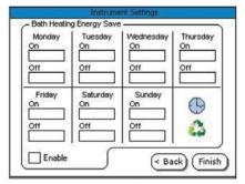
Control the heater/circulator by programming the on/off cycles for energy efficiency.
