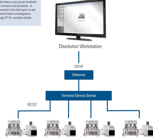
Dissolution Workstation Software can manage up to 4 systems from a single PC. Each PC on a common network can connect to a centralized database.
