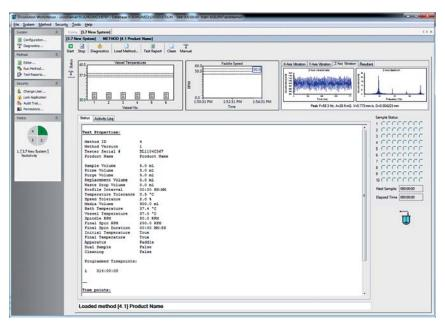
The Dissolution Software system status screen displays the activity of all systems in real time.
