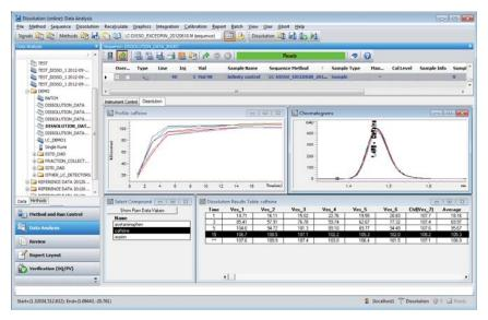
The run-time display shows profiles, actual values and the last spectra, as well as the status of instrument at a glance.
