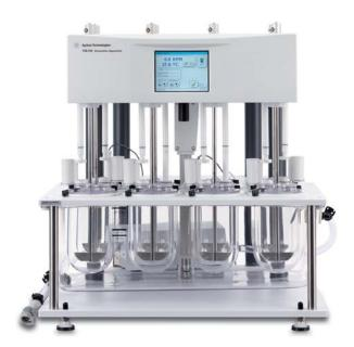
The 708-DS is easily configured for USP Apparatus 1, 2, 5, and 6 as well as Intrinsic Dissolution or Enhancer (Immersion) Cell use.
