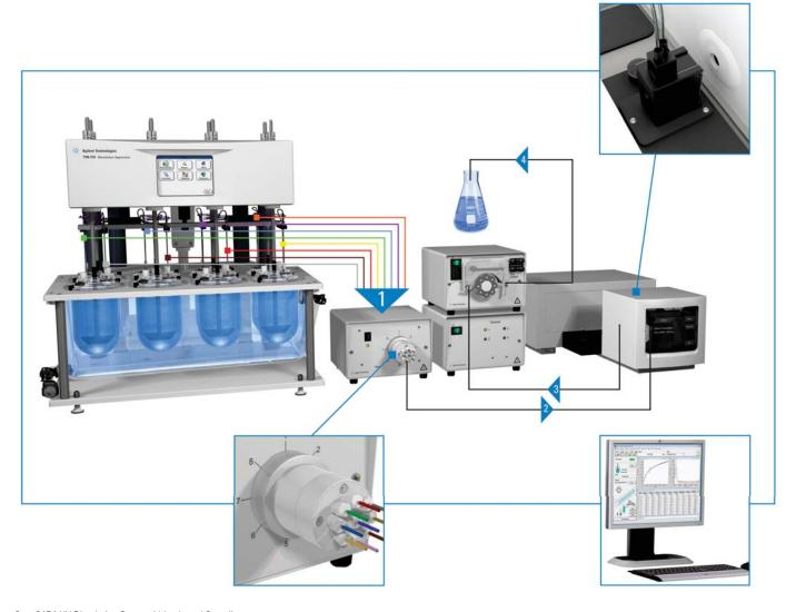
Cary 8454 UV Dissolution System: Valve-based Sampling
