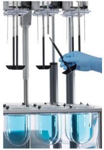
Upper shaft receptor and lower paddle piece
