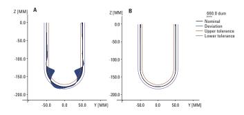
Variation in vessel shape between standard vessels tested by Agilent (A) and Agilent VF molded vessels (B), which exceed USP vessel tolerances. The center of the three lines indicates the ideal shape of the cylinder and hemisphere. The two lines drawn on both sides represent  $\pm$  0.3 mm from the center line.
