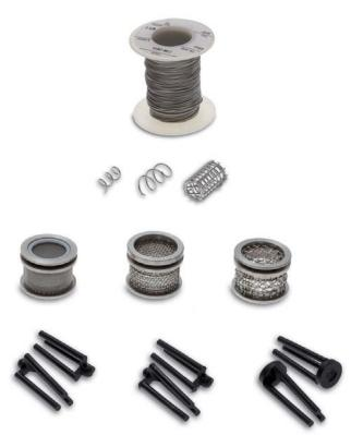
Capsule weight wire (top row), two versions of wire sinkers and a Japanese sinker (second row), mesh sinkers (third row) and 3-prong sinkers (fourth row)
