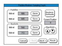
The ability to specify an exact depth for the manifold means that each sample is withdrawn from the same USP location within the dissolution vessel. This adds to the reproducibility and consistency for every test performed — a critical consideration for dissolution testing.
