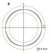
Variation in roundness between a standard vessel (A) and an Agilent VF molded vessel (B). The center of the three lines indicates the ideal shape of the cylinder and hemisphere. The two lines drawn on both sides represent  $\pm~0.3~\mathrm{mm}$  from the center line.
