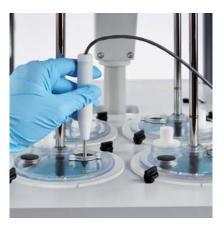
Manual temperature measurement using 708-DS temperature probe
