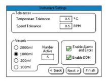
Specific settings and features within the 708-DS firmware such as tolerances, vessel volumes and alarms are easily adjusted to meet your laboratory's exact requirements.
