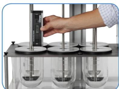
Horizontal & Vertical Levelling
