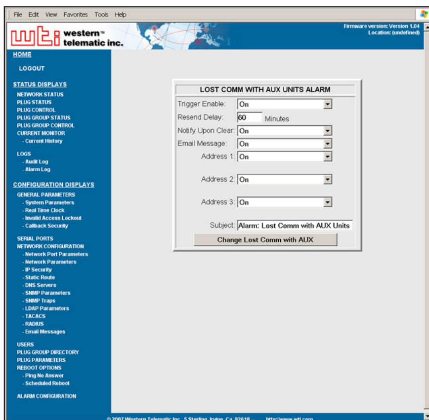
Figure 7.10: The Lost Communication with AUX Units Alarm Menu (Web Browser Interface)
