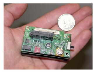
Fig. 4. Mica mote  $[2'' \times 1'' \times (3/4)'']$  with attached weather board module.
