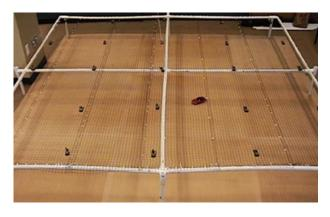
Fig. 8. Indoor sensor-based tracking testbed.
