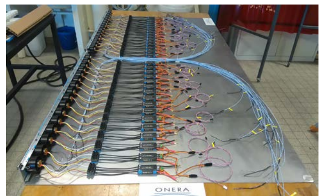
Fig. 15 – Ground test bench for propulsion architecture validation
