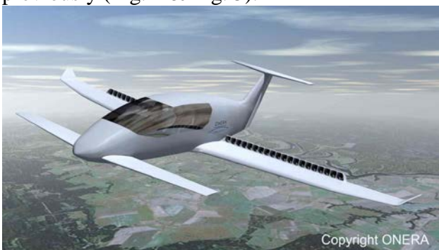
Fig. 4 Three-surface concept-plane with distributed EDF at the wing trailing edge
