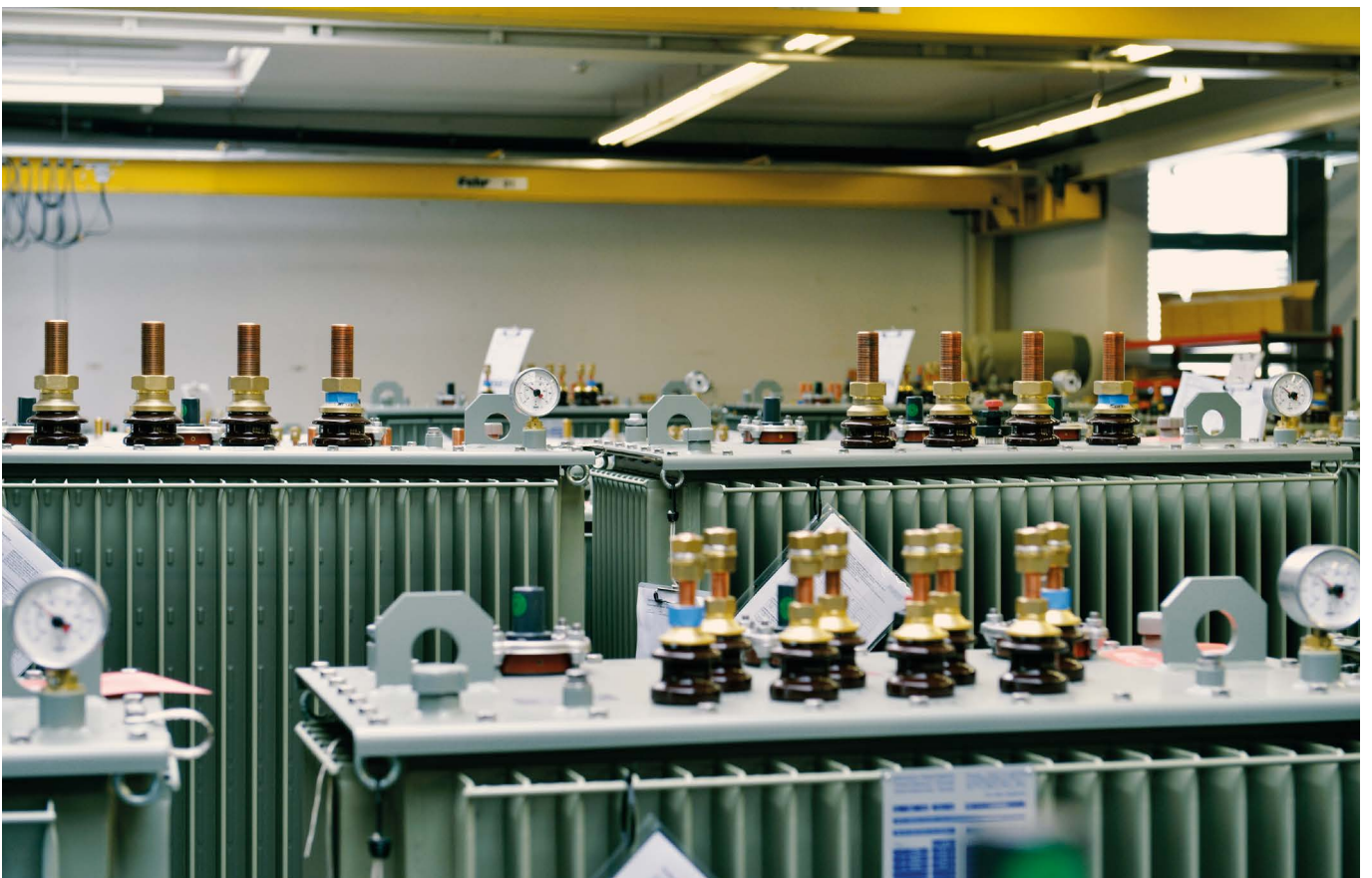
Distribution transformers prior to delivery
