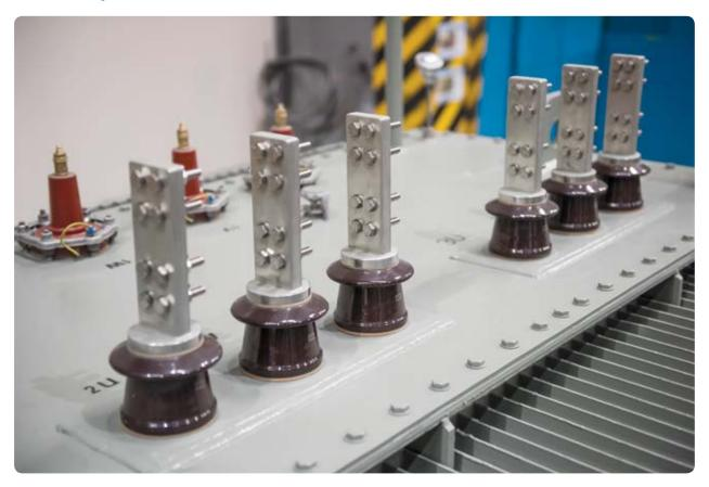
A Dual Voltage Transformer can be defined as the one capable of providing two types of voltages, i.e. if the two separate windings are connected in series, they will provide the sum of voltages supplied to the two coils and if the two windings are connected in parallel, then the net voltage will be decreased. These voltages can be switched within the transformer according to the type of output required by using a dual voltage switch.
