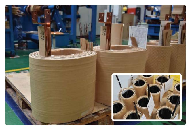
Both the primary and secondary windings are made of copper or aluminum. The primary voltage is directly wound on the secondary voltage winding, with insulating barriers and cooling channels between the two windings. Secondary voltage coils are rectangular wires or foil conductors. Primary voltage coils are round enamel wires, or rectangular paper insulated wires for high power ratings, or paper insulated round wires.
