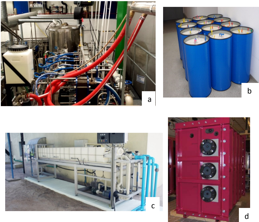
Figure 2.5. Semi-commercial MD modules from different suppliers. a) Xzero's AGMD pilot plant in Stockholm, b) Solarspring's spiral PGMD module [123], c) Memsys' VMD unit in Maldives [58], d) Memstill MD unit for a pilot system [124].
