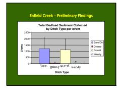
This pilot research indicates that suspended sediment and bedload are significantly higher from ditches that have been scraped and left exposed than from vegetated ditches.
