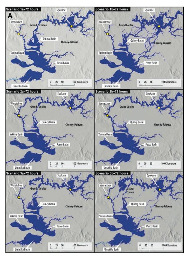
Figure 8 (*Continued on facing page*). (A) All scenarios 72 h after dam break, when flooding in each scenario is close to maximum stage in the large basins of Pasco, Umatilla, and Yakima. The variations in flooding between scenarios result from variations in the route taken to these basins. Between 72 h and 80 h, the stage in each basin begins to decline. Complete drainage of these basins through Columbia River Gorge takes many weeks.
