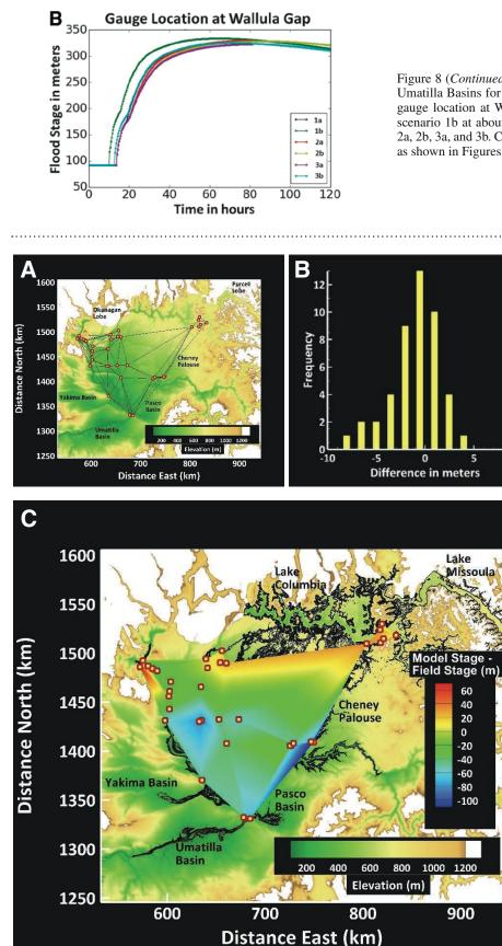
Figure 8 (*Continued*). (B) Variation in the rate of filling of Pasco and Umatilla Basins for each scenario tested, as determined with a model gauge location at Wallula Gap. Maximum stage is achieved first by scenario 1b at about 60 h, whereas 72 h is required for scenarios 1a, 2a, 2b, 3a, and 3b. Compare these results with the different paths taken as shown in Figures 6 and 7.
