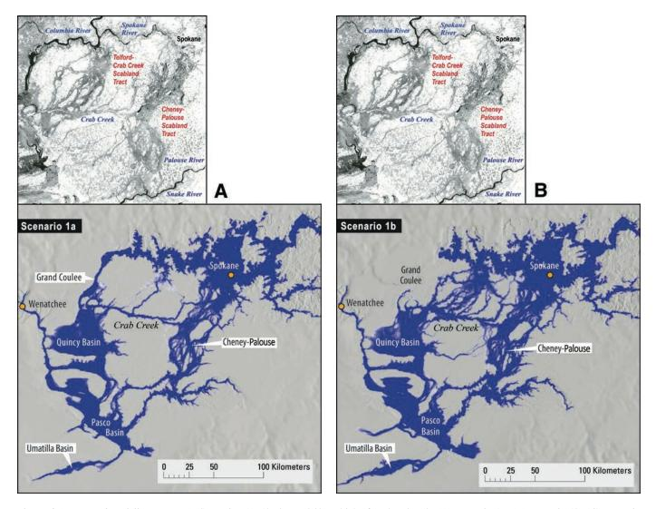
Figure 6 (*Continued on following page*). Scenarios 1a, 1b, 3a, and 3b at 23 h after dam break: (A) scenario 1a; (B) scenario 1b; (C) scenario 3a; and (D) scenario 3b. All flood Telford scabland. Only scenario 1b produces the broad extent of scarring visible in the satellite image above. Flooding of Telford scabland tract requires that the Columbia River valley is blocked, and maximum flooding of Telford scabland only occurs when flow into upper Grand Coulee is blocked.
