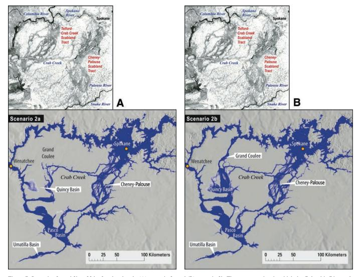
Figure 7. Scenarios 2a and 2b at 23 h after dam break: (A) scenario 2a and (B) scenario 2b. The two scenarios, in which the Columbia River valley is open, are required to match the field evidence for high water and erosion of Pangborn bar, the giant point bar forming the big bend in the Columbia River at Wenatchee. Scenario 2a floods Quincy Basin from the east; scenario 2b floods Quincy Basin from the west.
