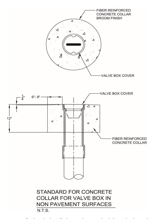
b. A concrete collar is to be installed around new and existing valve boxes in all asphalt surfaces. Collars shall be designed to the figure below.
