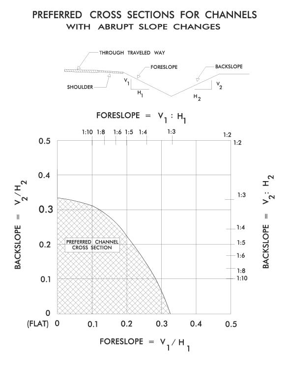
\*This chart is applicable to all Vee ditches, rounded channels with a bottom width less than 2.4 m (8ft) and a trapezoidal channels with bottom widths less than 1.2 m (4ft).
