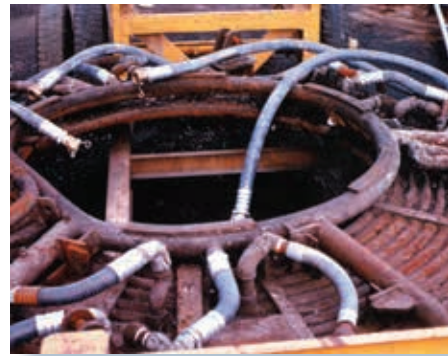
circulating water in an electric arc furnace cooling roof or furnace door
