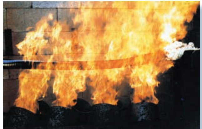
GSM BOP hose tested at 2000°F, 2,000,000 BTU's at 5,000 PSIWP.
