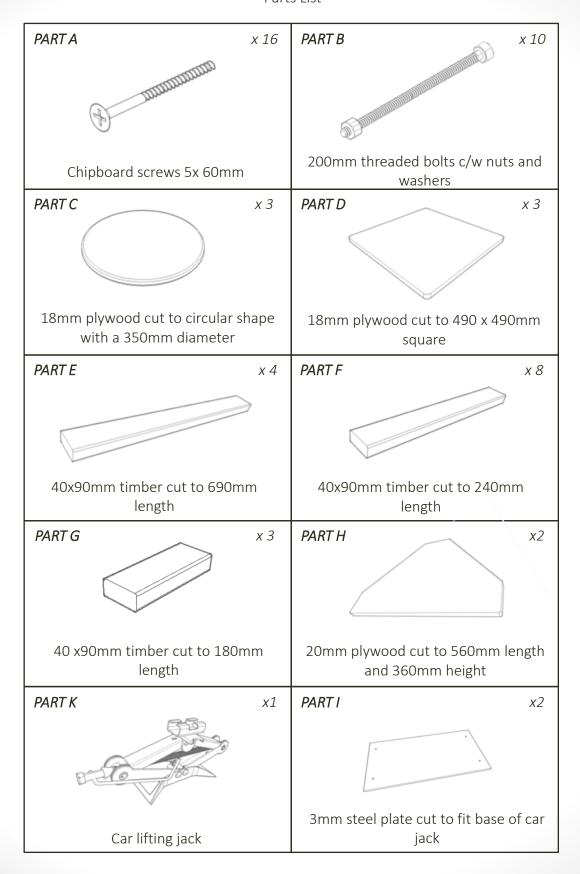
**Step 1**: You will need to assemble a rectangular frame using PART E and PART F. Lay out the base of your frame as shown below;
