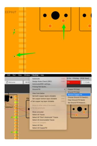
You can run the GPIO pins to the keyswitches on the bottom layer of the board to avoid having them cross the Pico's pads on the right side of the board, as well as the "keepout" area that is marked on the Pico's footprint indicating where there are pads, holes, and the USB connector pads to avoid.
