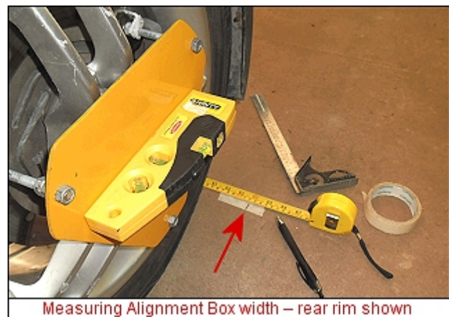
Marking laser width – rear wheel-rim shown
