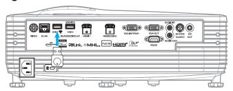
In order to utilize the embedded HDcast Pro Device Wireless Projection, you need to install the USB Wi-Fi dongle into the appropriate USB port on the back of the projector. Once the USB Wi-Fi dongle has been installed, HDCast Pro Device Wireless Projection are ready for use.
