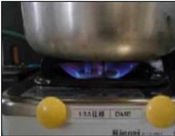
DME burning by cooking stove for natural gas
