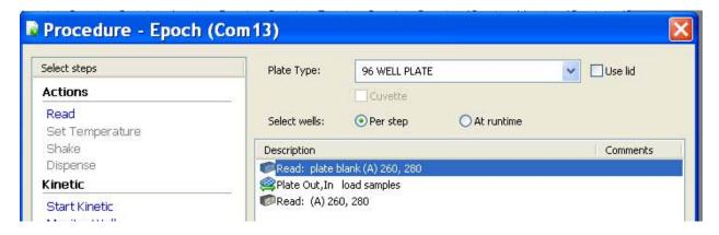
**Figure 9**: During microplate analysis of dsDNA samples the plate is first pre-read for blanking followed by sample loading and measurements at 260 and 280 nm using a standards Gen5 protocol.
