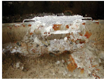
Figure 4-1 Corrosion at sacrificial anode; from left to right on attachment only, partially and completely consumed
