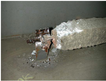
Figure 4-1 Corrosion at sacrificial anode; from left to right on attachment only, partially and completely consumed
