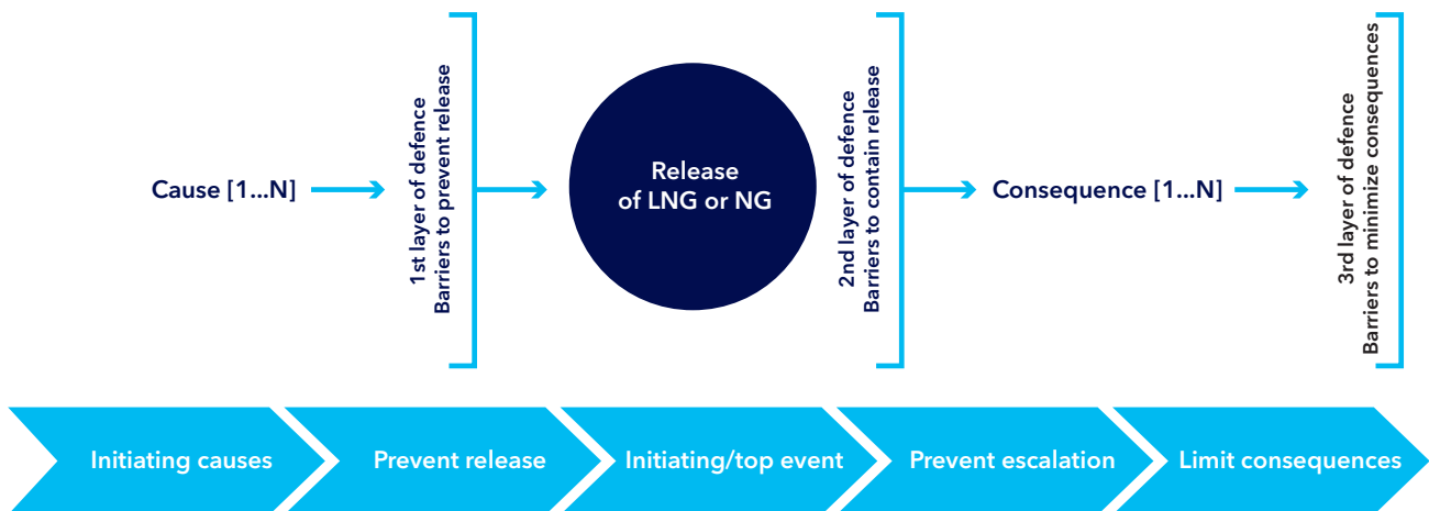
Figure 4-1 The three layers of defence illustrated in the bow-tie diagram /1/
