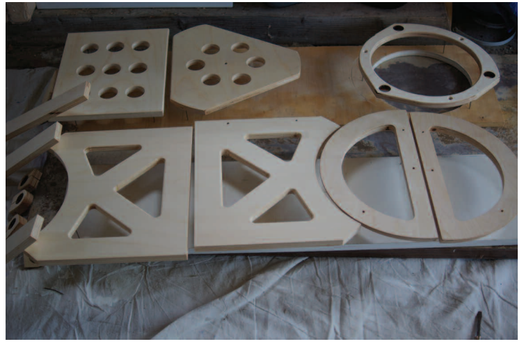
Image 5 - The main components of the kit are prepped for multiple coats of Ikea's user-friendly Behandla finish, a mixture of beeswax, linseed and tung oils.
