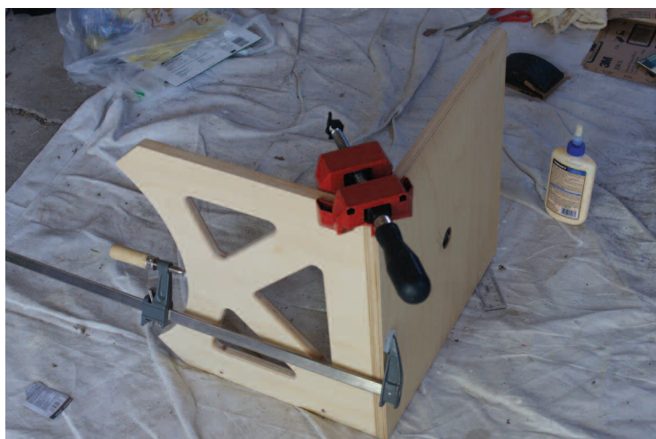
Image 7 - The rocker-box pieces are held in place with clamps as joint glue sets.
