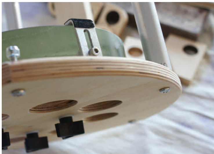
Image 8 - A universal primary-mirror cell from Compact Precision Telescopes (leftover from another project) was reused with the Dobstuff kit. Three holes were drilled in the base of the mirror box to pass the cell's collimation bolts.
