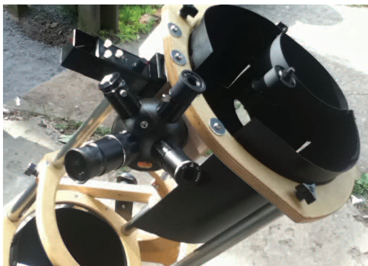
Image 10 - An eyepiece turret from a Vixen refractor carries an assortment of eyepieces on the f/4.2 version of the scope.
