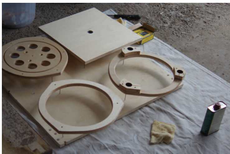
Image 6 - The author constructed a “bed of nails” for suspending the components as the newly-applied finish coats cured.
