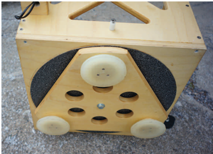
Image 2 - Brandon Geisel's (Tripodpads.com) tough, vibration-reducing urethane tripod pads were installed in place of more-standard Dob feet.
