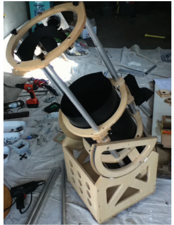
Image 1 - The author's Dobstuff 10-inch kit in f/4.2 configuration.
