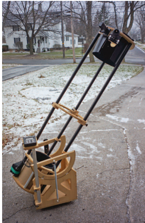
Image 12 - The f/7 version of the scope is significantly longer than its initial f/4.2 configuration, but remains sufficiently rigid to firmly hold collimation.
