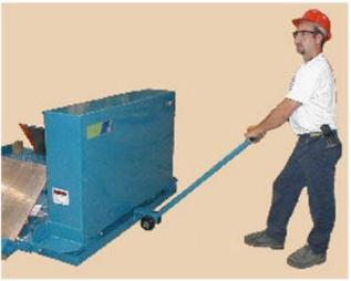
The unit is now portable. Never load the unit when casters are in use. Casters are for transporting the unit only.
