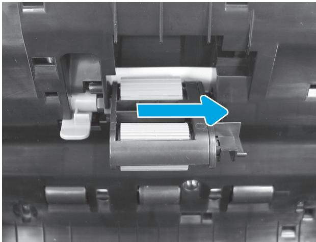
**EN** Rotate the roller assembly up into the holder (callout 1), and then slide the blue locking lever towards the back of the printer (callout 2).
