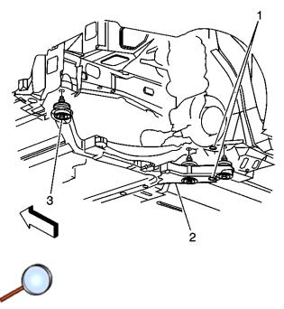
60. Remove the 6 frame to body mounting bolts (3).
