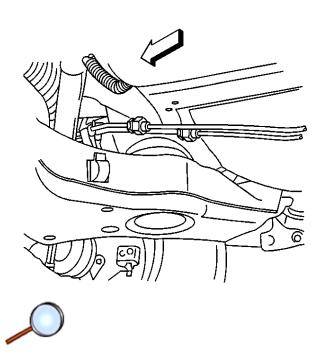
43. Connect the 2 rear brake pipes at the rear of the engine frame.
