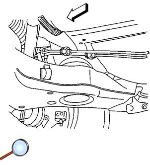
42. Disconnect the 2 rear brake pipes at the rear of the engine frame. Plug the open outlet ports to prevent fluid loss and contamination.
