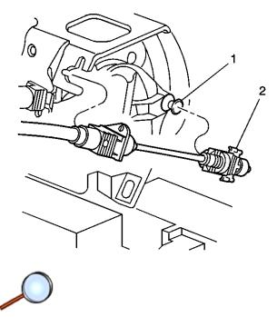
**Caution:** In order to avoid possible injury or vehicle damage, always replace the accelerator control cable with a NEW cable whenever you remove the engine from the vehicle. In order to avoid cruise control cable damage, position the cable out of the way while you remove or install the engine. Do not pry or lean against the cruise control cable and do not kink the cable. You must replace a damaged cable.
