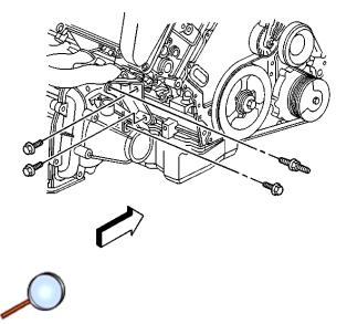
8. Install the 4 bolts securing the center transaxle brace to the engine and transaxle.
