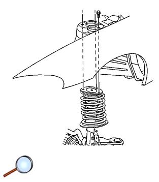
56. Install the right and left side strut tower bolts.
