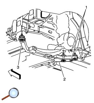
25. Position the engine/transaxle assembly under the vehicle.
