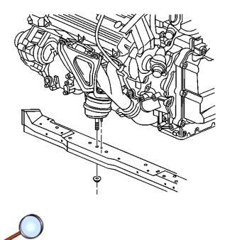
4. Install the nut securing the front engine mount to the front engine frame.
