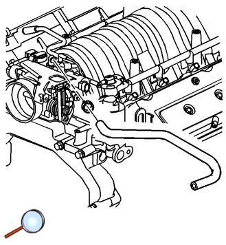
81. Connect the vacuum brake booster hose to the vacuum connection.
