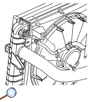
60. Install the upper transaxle oil cooler pipe retaining bolt to the fan shroud.
