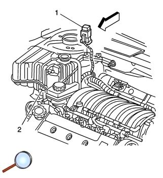
11. Disconnect the secondary AIR relay (1) from the relay bracket and secure to the top of the engine.
