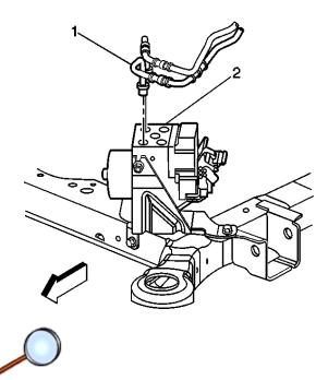
64. Install the 2 master cylinder brake pipes (1) to the BPMV (2) using the location recorded during the removal procedure.
