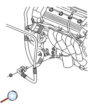
41. Connect the A/C discharge hose to the compressor.
