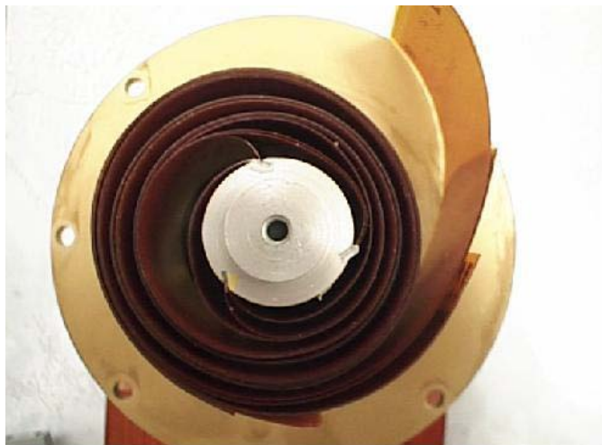
Figure 3: Wrapping Flexible Circuits of a Twist Capsule
