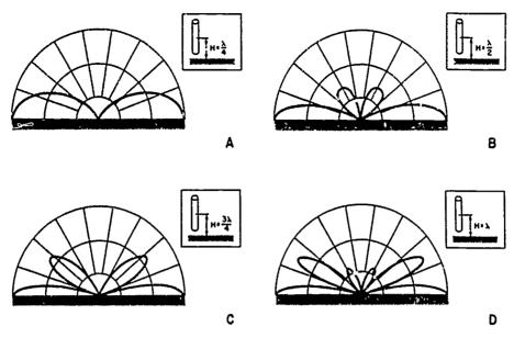
Fig 3-19. Vertical-plane radiation patterns produced by vertical half-wave antennas.
