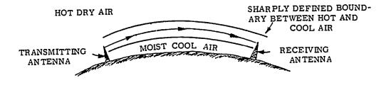
Fig 5-9. Transmission using the tropospheric duct.
