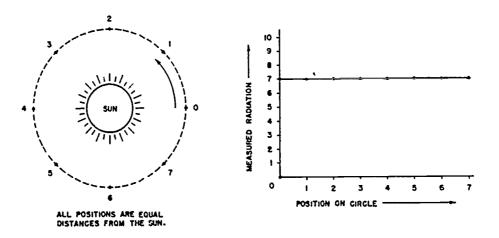
Fig 2-14. Isotropic radiation.
