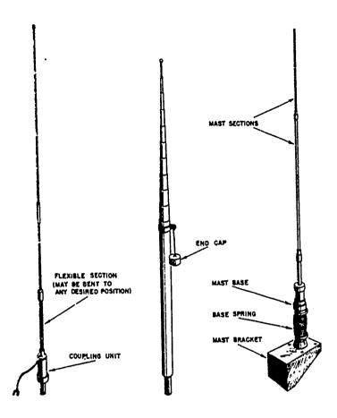
Fig 3-4. Common quarter-wave whip antennas.
