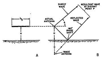
Fig 3-16. Reflection produced by ground plane.
