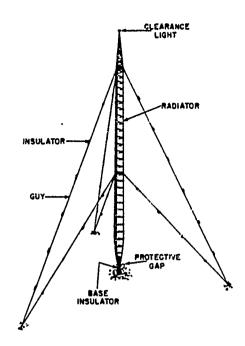
Fig 3-12. Insulated guyed-tower radiator.
