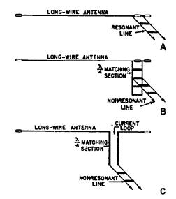
Fig 4-3. Feeding long-wire antennas.
