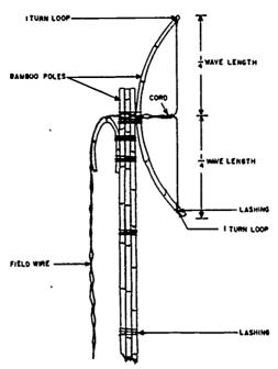
Fig 4-26. Improvised method of supporting a vertical half-wave antenna.
