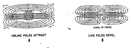
Fig 1-14, Lines of force between unlike and like poles.
