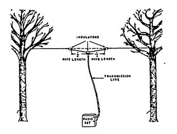
Fig 4-24. Improvised half-wave antenna.
