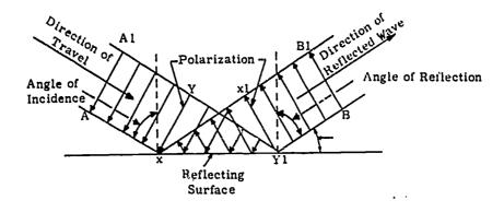
Fig 5-2. Reflection of a radio wave.
