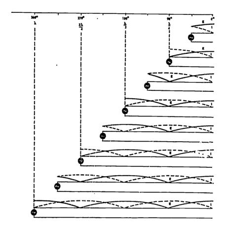
Fig 2-21. Voltage and current on an open transmission line.
