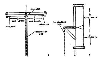
Fig 4-25. Improvised vertical and horizontal half-wave antennas.
