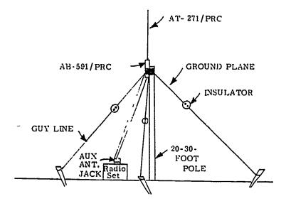
Fig 4-29. Ground plane antenna improvised by using the AN/PRC-25 antenna.
