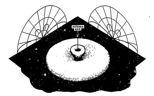
Fig 3-20. Radiation pattern of a vertical half-wave antenna located a half wavelength above ground.
