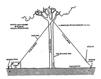
Fig 4-27. Improvised half-rhombic antenna.
