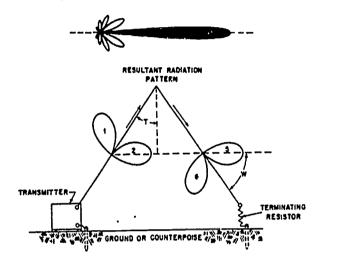
Fig 4-10. Terminated half-rhombic antenna and resultant radiation pattern.
