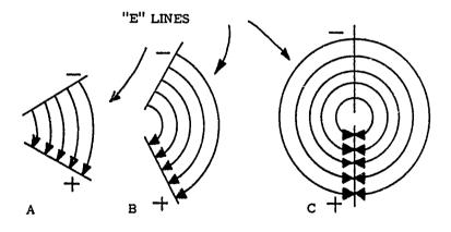
Fig 2-6. Open electric field.
