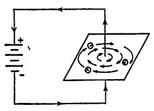
Fig 2-1. Magnetic field about a current-carrying conductor.
