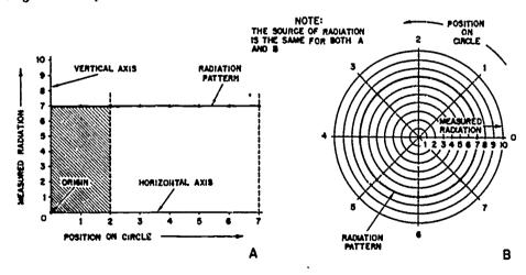
Fig 2-16. Comparison of rectangular- and polar-coordinate graphs for an isotropic source.
