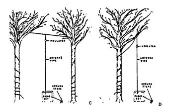
Fig 4-23. Improvised vertical antennas.
