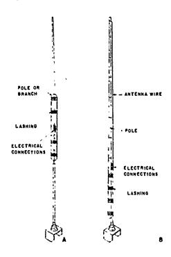
Fig 4-21. Whip antenna repair.
