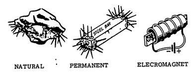
Fig 1-8. Three types of magnets.
