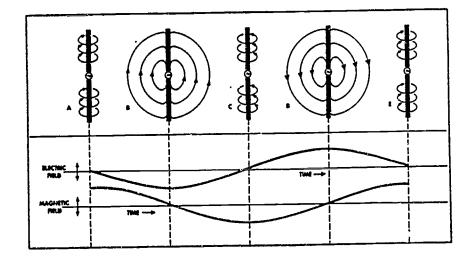
Fig 2-9. Comparison of the "E" and "H" fields.
