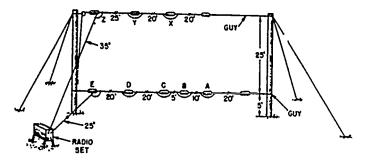
Fig 3-8. Inverted-L antenna with counterpoise.
