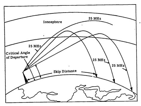
Fig 5-19. High-frequency wave at various angles of departure.
