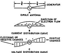
Fig 2-10. Voltage and current distribution of a dipole antenna.
