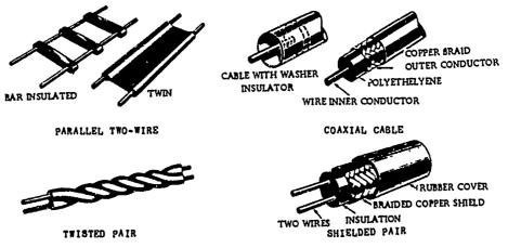
Fig 2-23. Four general types of transmission line.
