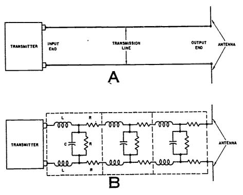
Fig 2-20. A transmission line and its equivalent circuit.
