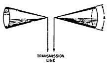
Fig 3-24. Simplified conical antenna.
