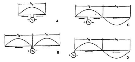
Fig 4-1. Harmonically and nonharmonically operated antennas.
