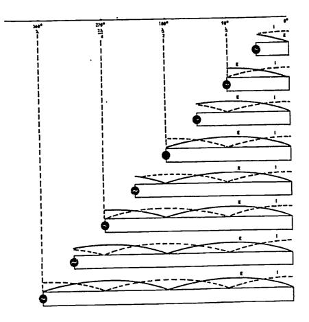
Fig 2-22. Voltage and current on a shorted transmission line.
