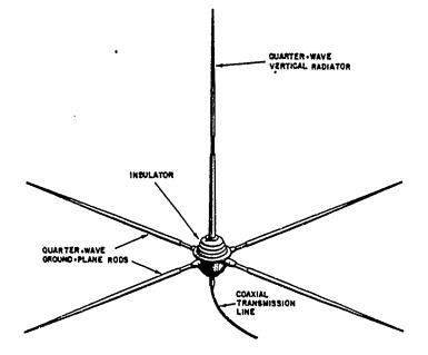
Fig 3-5. Typical ground plane antenna.
