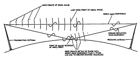
Fig 5-7. Comparison of the direct and the ground-reflected wave.
