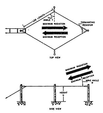
Fig 4-11. Basic rhombic antenna.
