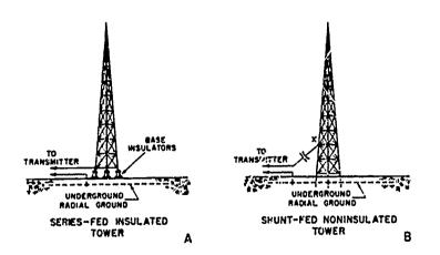
Fig 3-13. Series- and shunt-fed tower radiators.
