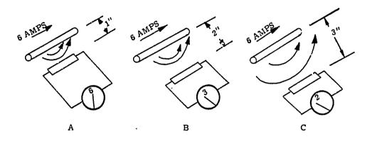
Fig 2-7. Effects on the "E" field as the distance from the conductor is varied.
