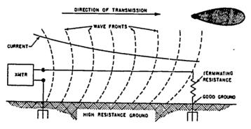
Fig 4-4. Beverage or wave antenna.
