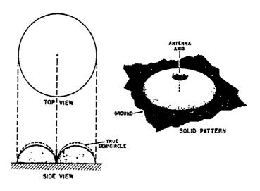
Fig 3-3. Radiation pattern of a quarter-wave antenna.
