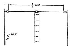
Fig 3-14. Basic Hertz antenna.
