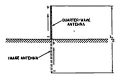
Fig 3-1. Quarter-wave antenna connected to ground.
