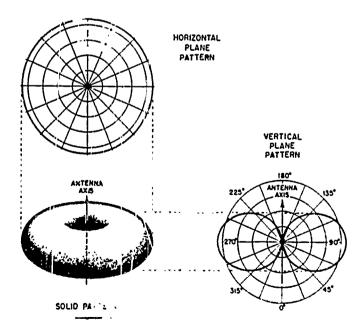
Fig 3-15. Iladiation pattern of a dipole (half-wave) antenna.
