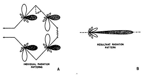
Fig 4-12. Formation of the rhombic radiation pattern.
