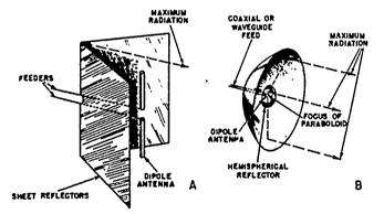
Fig 3-26. Special reflectors for half-wave antennas.
