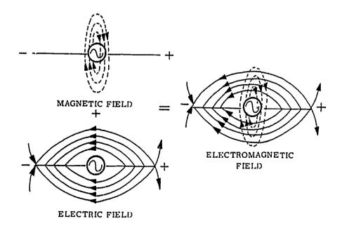
Fig 2-8. Components of the electromagnetic field.
