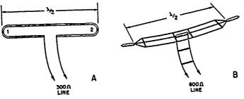
Fig 3-22. Folded-dipole antenna.
