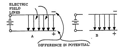
Fig 2-5. Electric field between capacitor plates.
