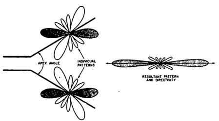
Fig 4-6. Formation of the V antenna radiation pattern.
