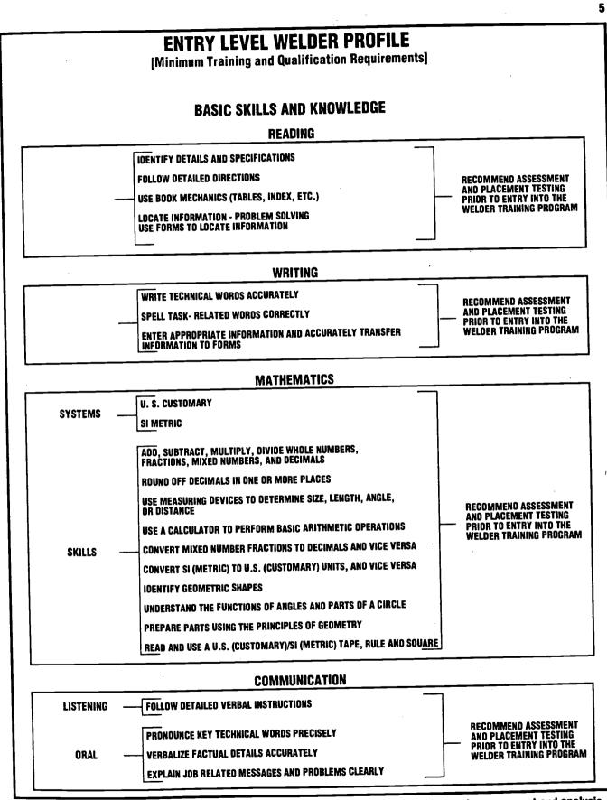
Figure 1— Entry Level Welder Profile. This information was developed as a result of a needs assessment and analysis from a national survey distributed to a mailing from the roles of AWS membership.
