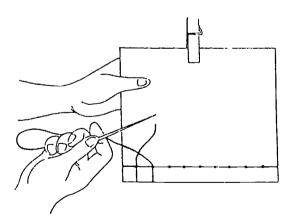
Continue until the last hole is reached. Retrace steps so that the spaces between the holes are filled in (down through one hole and up through the other.)
