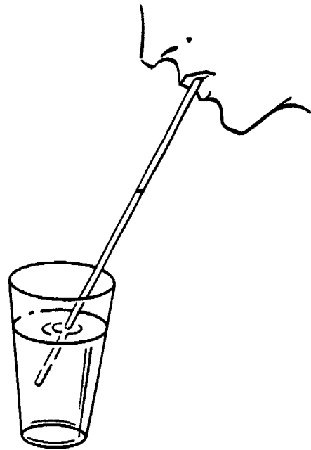
Figure 4. Partial vacuum produced by suction.
