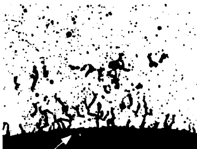
A INTERGRANULAR CORROSION
