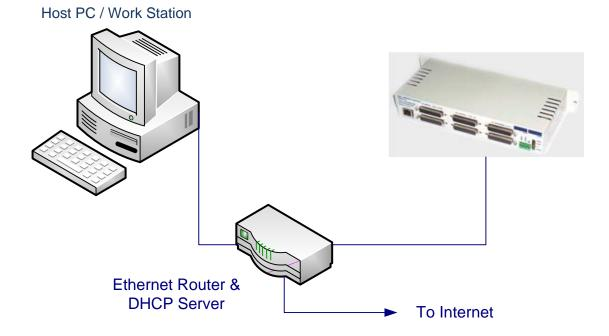
The figure above shows a basic setup using a router on your network. Connect the Ethernet cable from the J1- Ethernet port of the DSPMC board to the DHCP server/Router. Connect another Ethernet cable from the DHCP Server/Router to the PC. The DHCP server dynamically assigns IP address both to the PC as well as to the DSPMC board, and therefore completes the network setup without requiring any intervention from the user.
