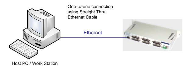
The PC IP Address can be configured manually in windows XP as follows. For other operating systems, please consult the respective user guides for changing the IP address.
