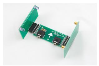
The two cables from the projectile sensor are plugged into the Sensor 1 and Sensor 2 ports. Sensor 1 would be the first sensor in the path of the projectile and Sensor 2 would be the second senor as written on the sensor printed circuit board. The flash(s) are connected to the Camera/Flash 1 and/or the Camera/Flash 2 ports.
