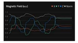
Figure 6: Mag Norm fluctuates when moving
