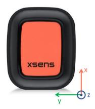
Figure 12: Xsens DOT sensor coordinate system
