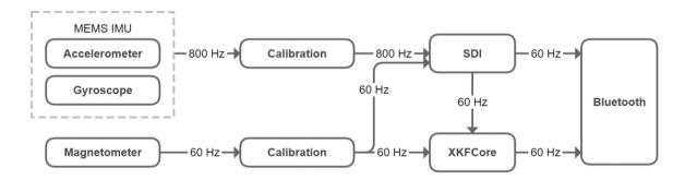
Figure 7: Xsens DOT signal processing architecture
