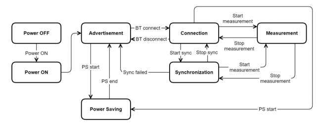
Figure 8: Xsens DOT state transition diagram
