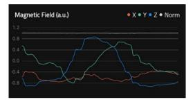
Figure 5: Mag Norm is constant while moving
