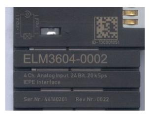
Fig. 34: ELM3604-0002 terminal with unique ID number (QR code) 100001051 and serial/ batch number 44160201
