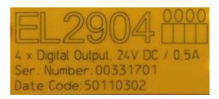
Fig. 33: EL2904 IP20 safety terminal with batch number/ date code 50110302 and unique serial number 00331701
