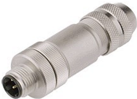
Fig. 25: M12 connector, 4-pin, IP67, for field-assembly, d-coded
