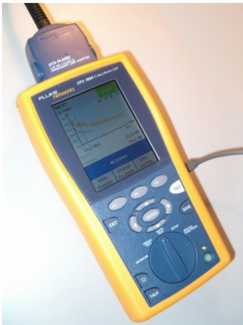
Fig. 34: Example illustration of a cable certifier
