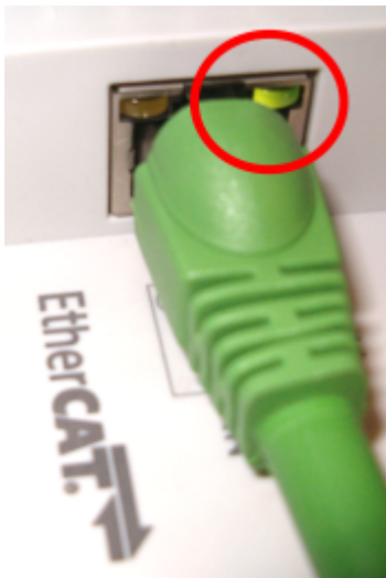
Fig. 33: Link LED on Ethernet devices
