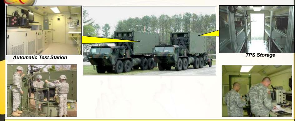
NGATS is a highly mobile, rapidly deployable, general-purpose, reconfigurable automatic test system which directly supports testing and screening of Army weapon systems to maintain their readiness to shoot, move, and communicate. Designated to replace Direct Support Electronic Systems Test Set (DSESTS), Base Shop Test Facilities (BSTF) versions 3 and 5, and other legacy automatic/automated off-platform test equipment currently used by the Army.
