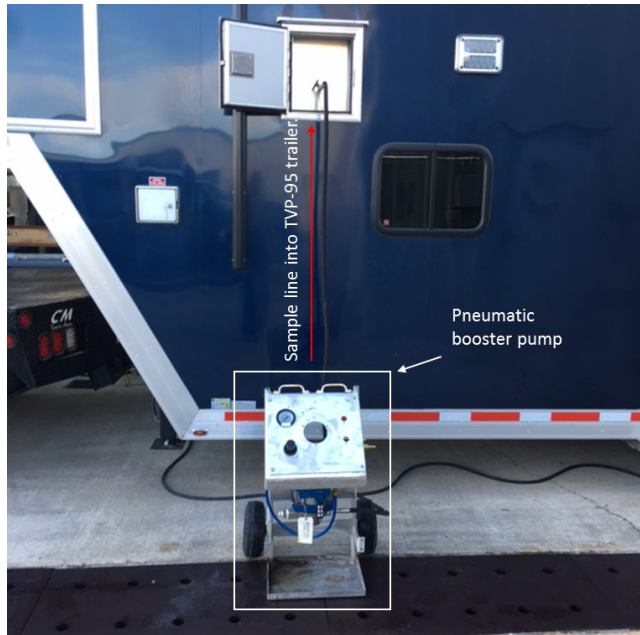
Figure 4-4. Pneumatic booster pump that raises sample to 500 psi prior to injection into TVP-95 trailer. Photo provided with permission from CoreLab.
