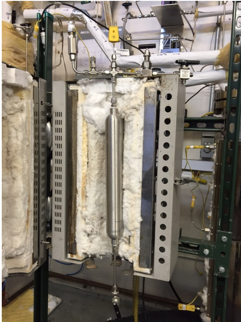
Figure 4-15. Photograph of PVT cell inside clamshell heater, reproduced with permission from University of North Dakota EERC.
