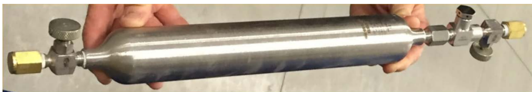
Figure 4-7. Representative GPA 2174 water displacement cylinder. Photo by David Lord and reproduced with permission from Intertek.
