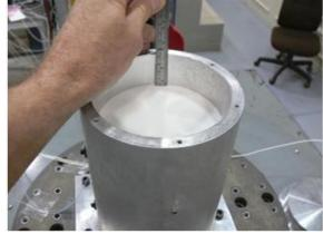
High Density Perlite exhibited compaction in the range of 13-17% after X-axis vibration (left) and Z-axis vibration (right). Photographs of typical results.
