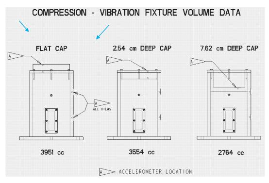
Vibration test fixture showing accelerometer locations and compression levels by different caps.
