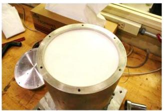
K1 Glass Bubbles after X-axis vibration, 4% void (left) and after Z-axis vibration, 2.5% void (right). Photographs of typical results.
