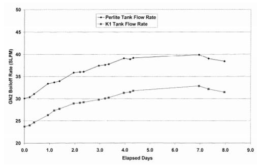
NER comparison test #1: perlite vs. K1 bubbles
