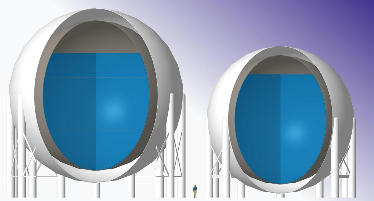
Scale comparison of new 4,700-m³ storage tank (left) and Apollo-era 3,200-m³ tank (right)
