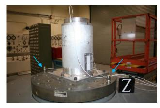
Lateral (X,Y) vibration test fixture with arrows pointing to response accelerometers (left photo) and vertical (Z) vibration test fixture with arrows pointing to control accelerometers (right).
