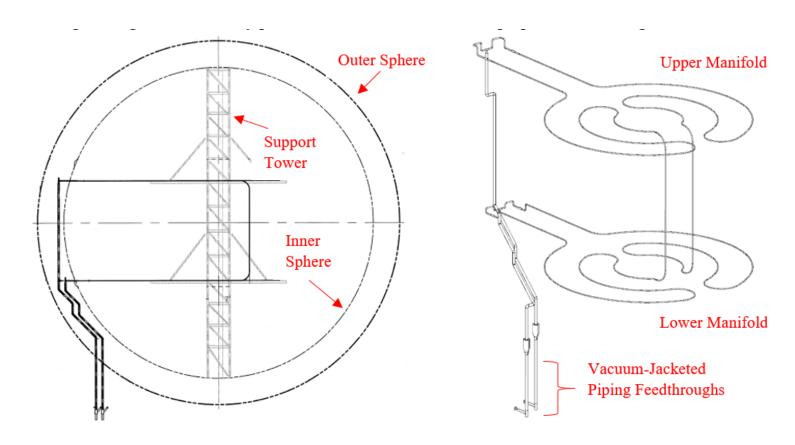
Heat exchanger configuration inside the sphere (left); 3D view of refrigerant feedlines and manifold (right)
