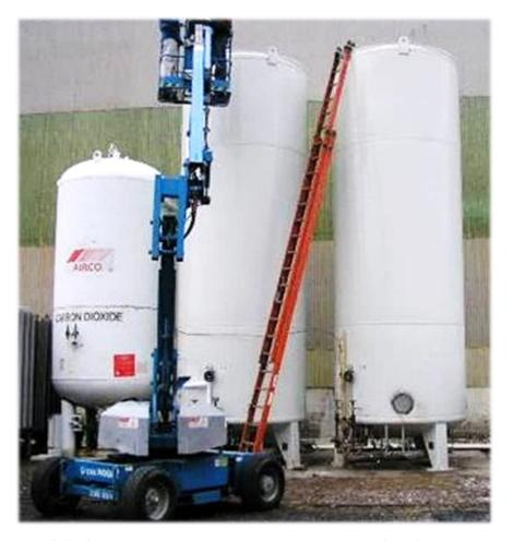
Field demonstration testing of standard VT-250 22,700-L (6000-gal) tanks located outside the ACME facility for identical environmental conditions
