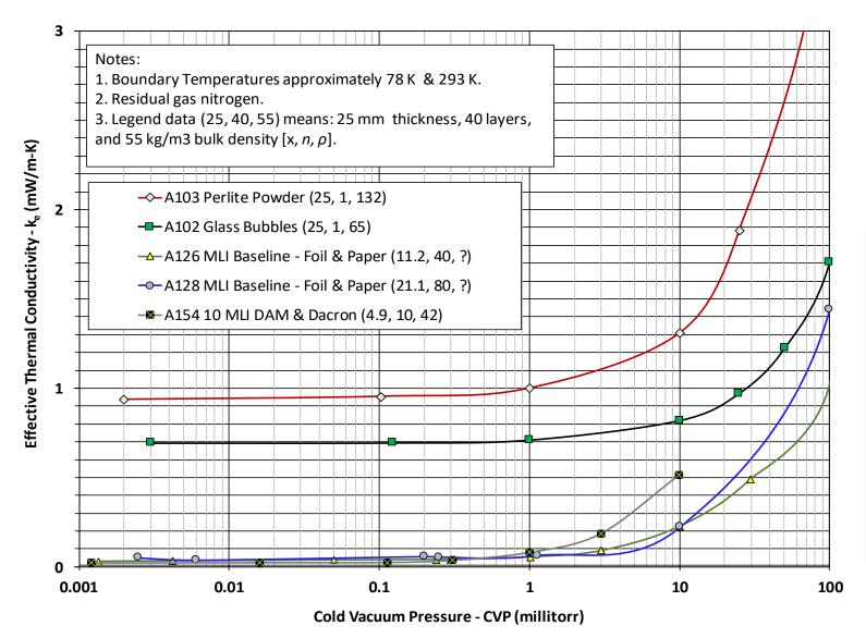
Glass Bubbles thermal performance data in comparison with other materials/systems (Cryostat CS-100)
