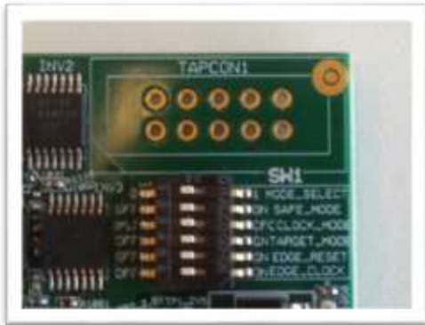
Picture 3: DIP Switch SW1 location
