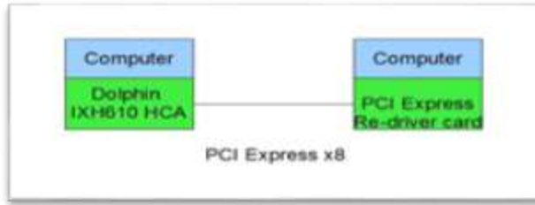
Illustration 3: IXH610 Adapter card used to connect to a remote host using a re-driver card.
