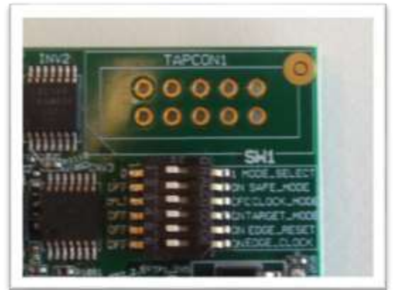
Picture 1: DIP Switch SW1 location
