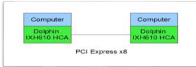
Illustration 4: IXH610 Adapter card used to build a two node configuration.
